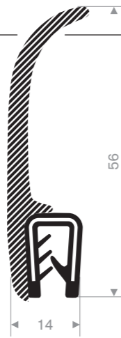
Item code 3924500876 Quality Full- + Sponge rubber EPDM Clamping range 1-3 mm Colour Black Length 25 meters
