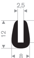
Item code 3921101201 Black Item code 3921101202 Grey Quality EPDM Hardness 70° Shore Length 100 meters
