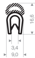
Item code 3924500817 Quality PVC + Sponge rubber EPDM Clamping range 1,5-3 mm Colour Black Length 50 meters
