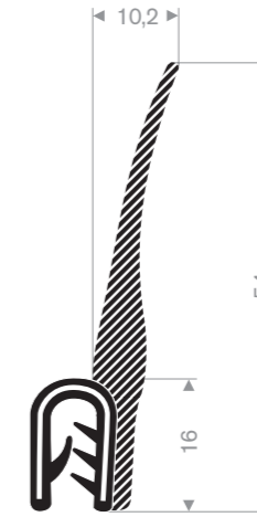
Item code 3924500910 Quality Full- + Sponge rubber EPDM Clamping range 1,5-5 mm Colour Black Length 25 meters
